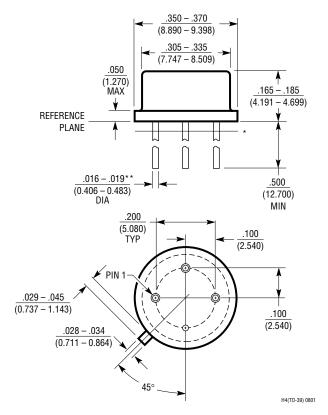
\*LEAD DIAMETER IS UNCONTROLLED BETWEEN THE REFERENCE PLANE AND .050" BELOW THE REFERENCE PLANE
